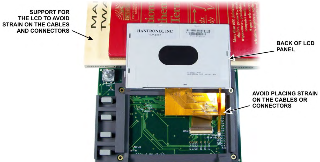
Figure 23. Removing LCD Panel from Rubber Key Matrix.
