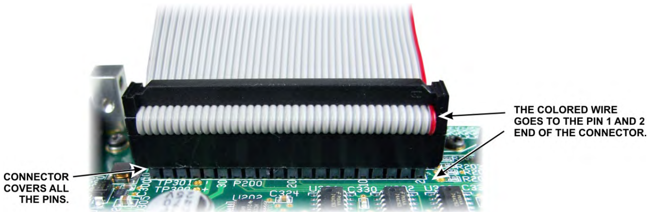
Figure 19. Mating the 40-pin Connectors.
