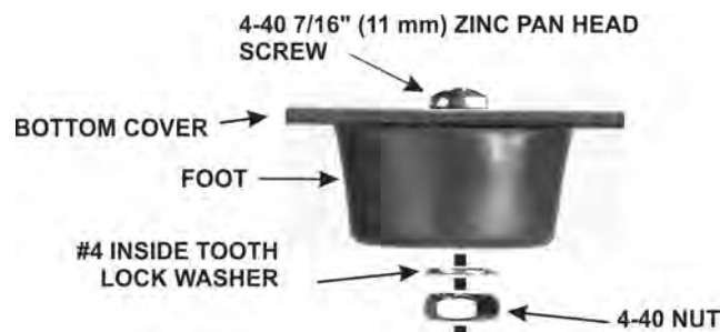
Figure 8. Installing Rear Feet.
